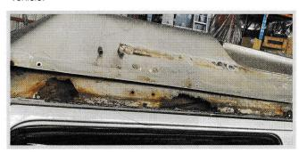
The damage had been caused by a previous owner pop riveting along the passenger side of the pop-top base through the fibreglass into the body of the roof of the van. The rivets were aluminium and of course through a process of electrolysis had caused the rust problem.
