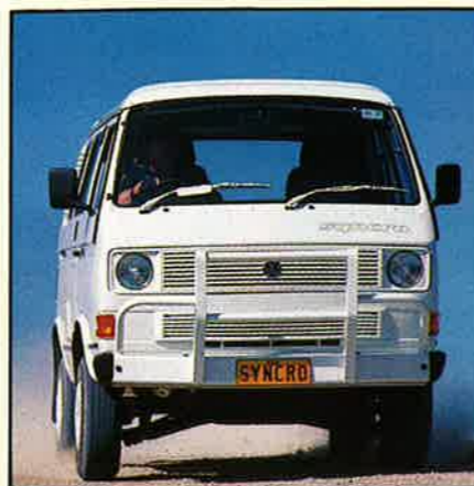
The Syncro is a well-balanced vehicle which handles fast dirt roads well due to the viscous coupling.
