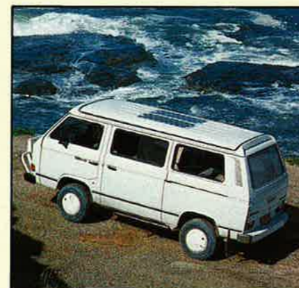
Solar panels on pop-top roof recharge batteries.
